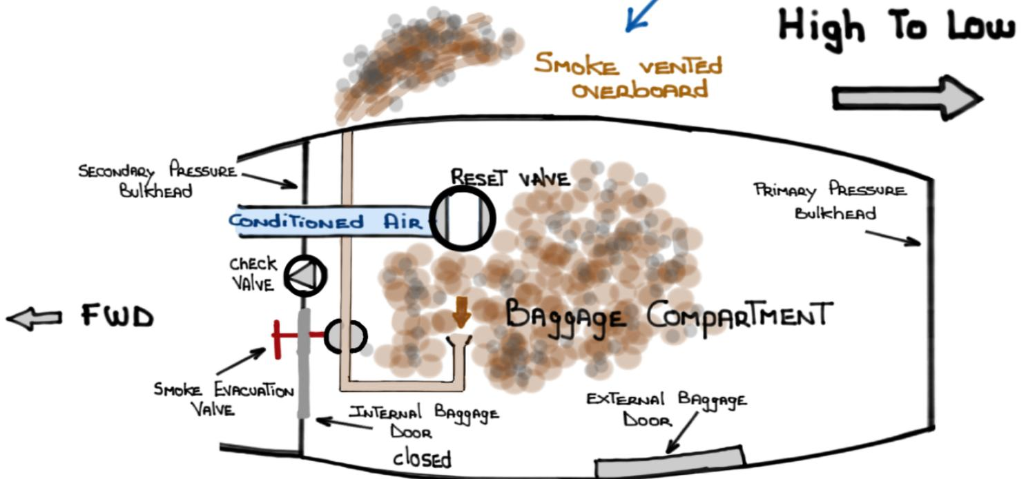
SMOKE IN THE CABIN CAN ALSO BE VENTED OVERBOARD BY PARTIALLY OPENING THE INTERNAL BAGGAGE DOOR
