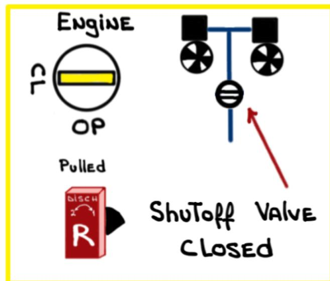
② Shuts off Hydraulic fluid DOWNSTREAM FROM RESERVOIR
